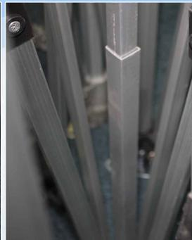
Small inner spring so it fits into the Centre pole, no way to see if it fails on the job, not strong enough to do the job properly for a heavy duty frame
